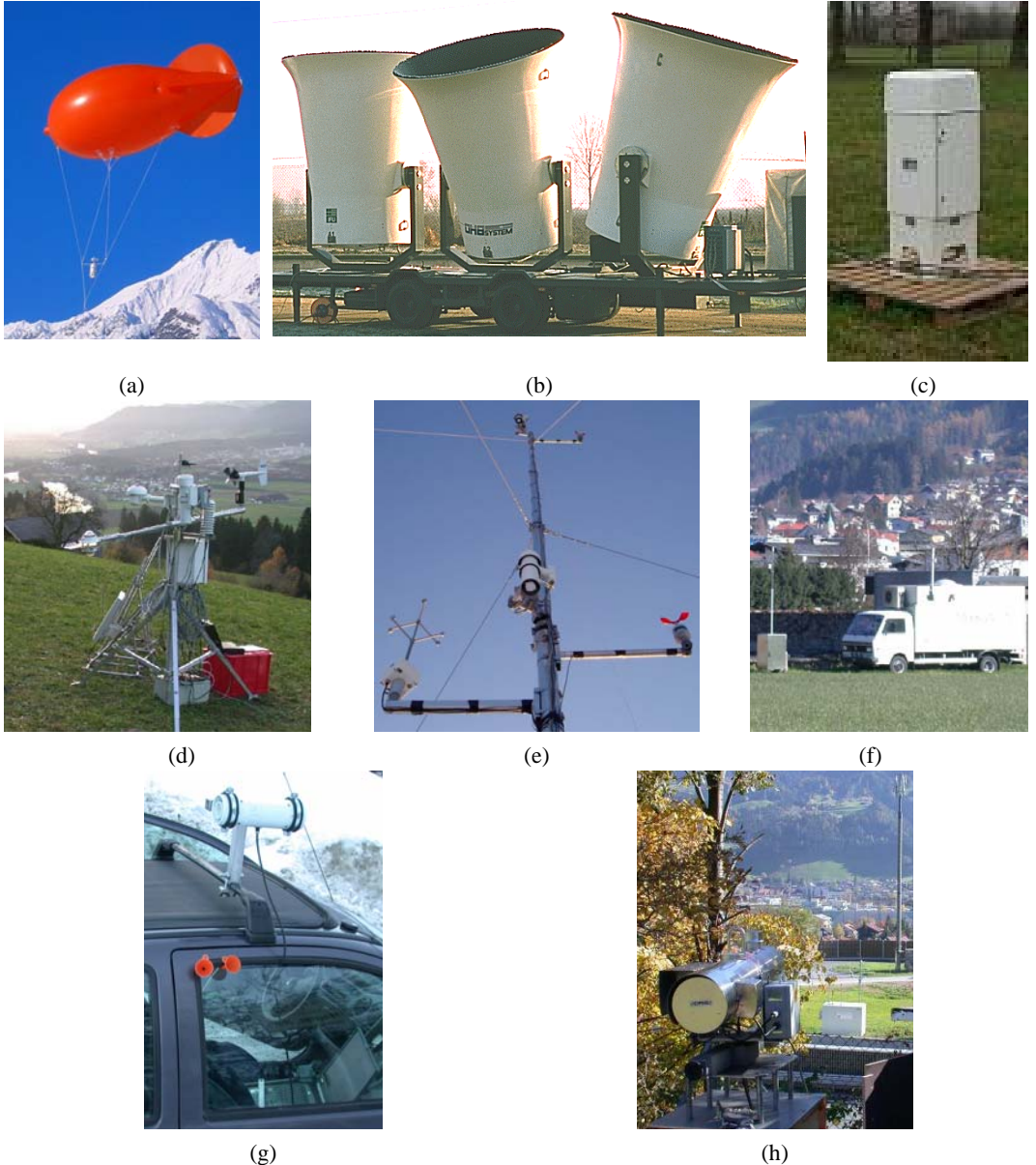
Fig. 7.4: Selected images of the measurement devices: (a) Tethersonde balloon and meteorological sonde; (b) Sodar; (c) Ceilometer; (d) Automatic Weather Station (AWS) at Arzberg; (e) AWS at basic station Schwaz (10 m mast); (f) air pollution measurement van and separate (g) PM10 unit (left) and mobile car platform (right); (h) Differential Optical Absorption Spectrometer (DOAS) looking across the motorway
