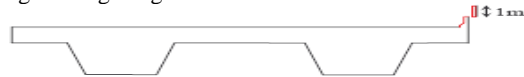
Fig. 5.15c Geometry of the platform with a 2 m barrier having a horizontal slit
