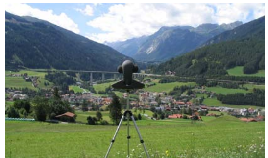
Fig. 5.8 Alpine valley with a motorway on a viaduct (Brenner route near Steinach/Austria) and an artificial head microphone in the foreground. Photo: P.Lercher.
