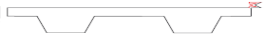
Fig. 5.15b Geometry of the platform with the absorbing sigma-shaped 1 m high edge barrier
