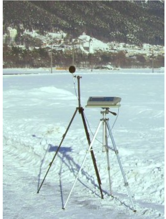
Fig. 5.11 Sound level meter (Norsonic 121) during the ALPNAP field campaign in the Lower Inn valley (Photo: M.Kästner).
