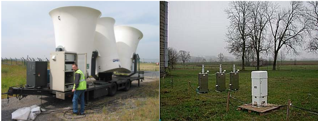
Fig. 3.12 Long-range Sodar (left), ceilometer (right; white device with aerosol samplers in the background).
