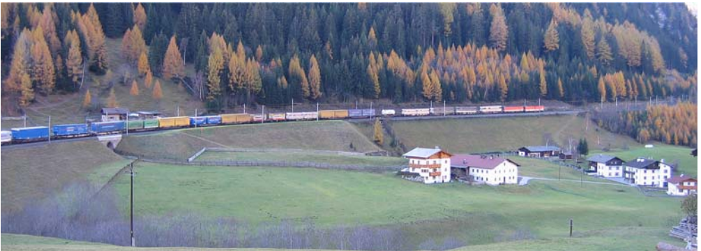
Fig. 2 A long freight train climbs up the track towards the Austrian-Italian border. It carries swap bodies and trailers and thus symbolises modern intermodal transport.
