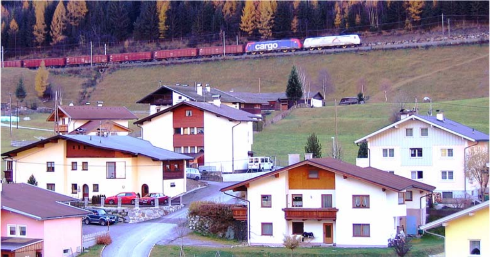
Fig. 4 Three electric locomotives, two pulling and one pushing, are necessary to move the rumbling waggons of this heavy freight train up the steep ramp towards the Brenner pass nearby the village of St. Jodok/Tyrol.
