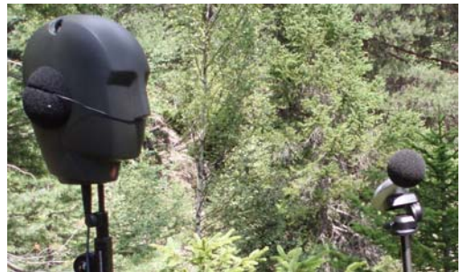
Fig. 17 A binaural artificial head microphone (left) and a monaural microphone (right) are listening the traffic noise in a recreation area of the French Maurienne valley. Both sensors are wind protected with foam.
